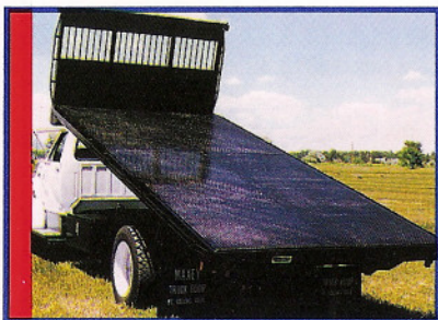
18' Lumber bed with treadplate floor
