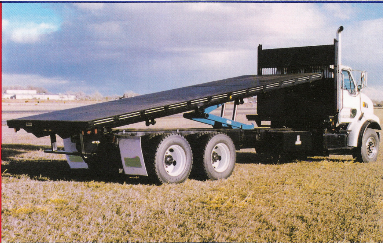
24' Lumber bed with 24" stationary drome headboard, treadplate steel over wood floor.
