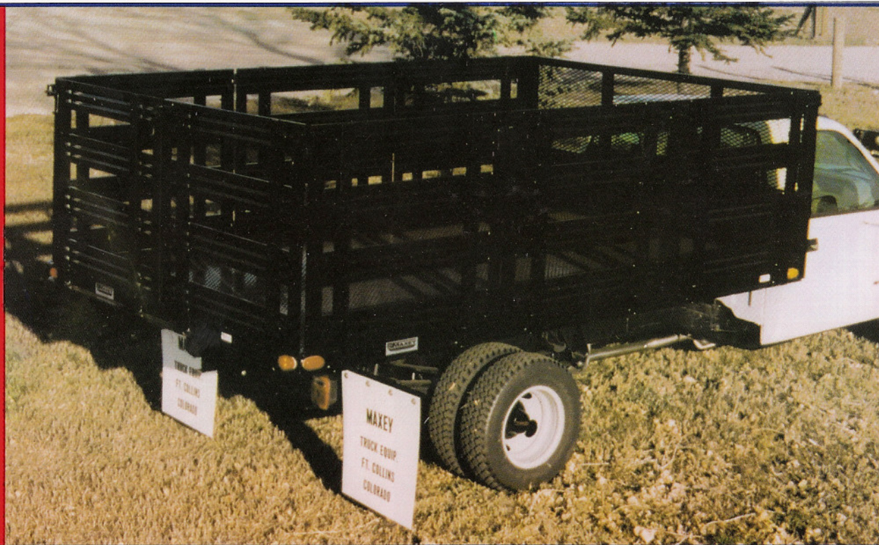
12' heavy duty platform with 1/8" treadplate floor, 40" headboard and 40" city stake sides
